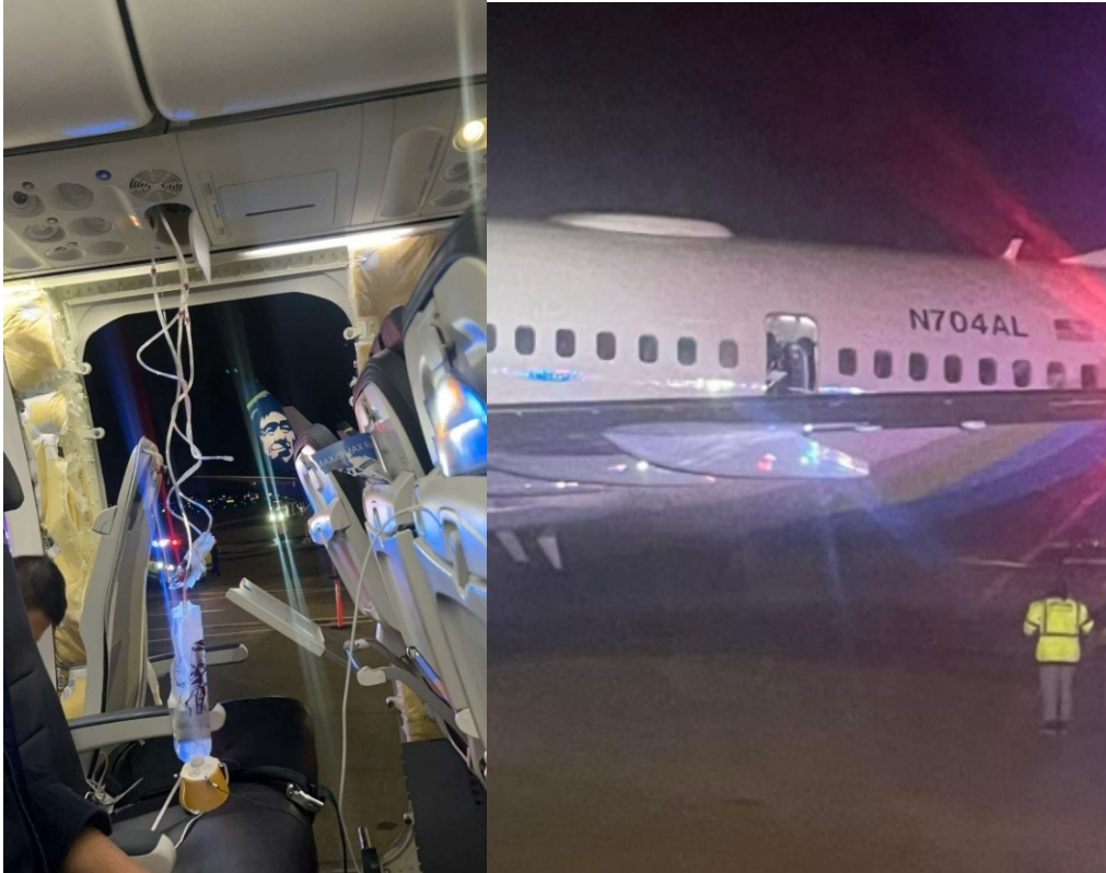
Figure 1. Photos of the location of the missing MED plug. (Source: left photo provided by a passenger. Right photo provided by media.)
